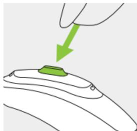
**A long push** (3 seconds) is used to switch the CROS device on/off.
